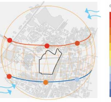
The West is the hottest side, so the design must limit the radiation that enters through this side, while still allowing for wind to enter during Habagat.
